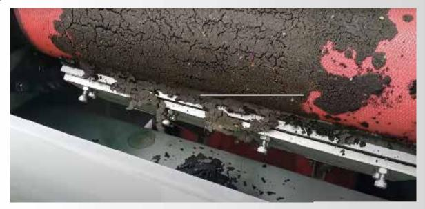
In contrast to mechanical dewatering, the MP-EDW does not put mechanical pressure on the material. The belt and drum serve purely as transportation mechanism and simultaneously function as electrodes, to which electrical voltage is applied. All moisture loss is achieved through electrophoresis and electroosmosis, driven by the passage of electric current.
