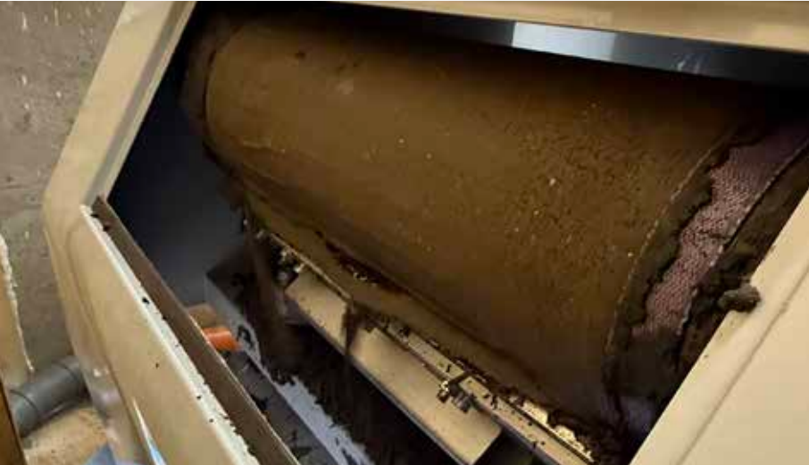
Dewatered cake coming from MP-EDW
